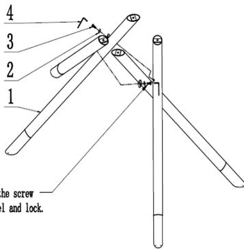
Put the screw into the screw hole adjust the level and lock.
