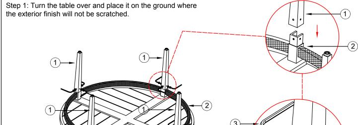
Step 2: Align the screw holes of the table legs with the screw holes of the table top, insert flat washers(5) and screws(4) into each hole, once the screws are in place, tighten the screw until firmly attached with the wrench provided.
