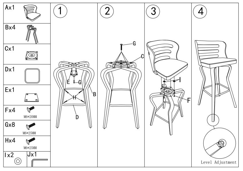
Note: (1) Lightly tighten the screws indicate on Step 1.
