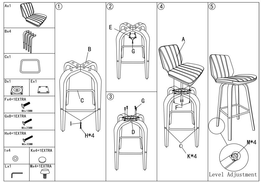
Note: (1)Lightly tighten the screws indicate on Step 1 & 2.
