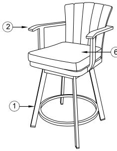
Step 2: Align the screw holes of the chair leg with the screw holes of the seat, insert flat washers(5) and screws(4) into each hole, once the screws are in place, tighten the screw until firmly attached with the wrench provided.
