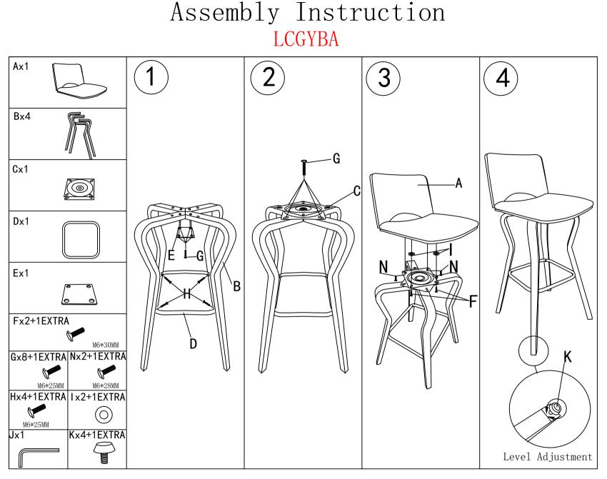
Note: (1) Lightly tighten the screws indicate on Step 1.
