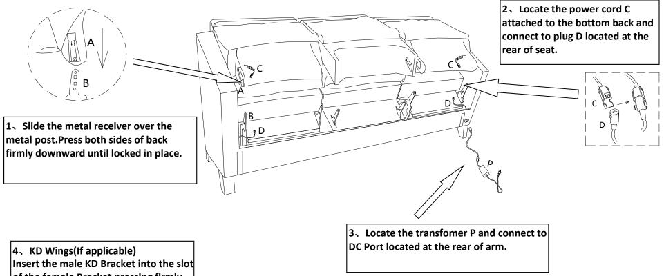
of the female Bracket pressing firmly downward until the frame is tight.
