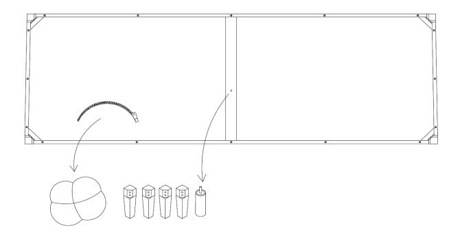
STEP 2. Attach the leg to wood frame using bolt and washer, with allen wrench Now tighten all bolts securely. Caution: do not over thighten bolts as damage could occur.
