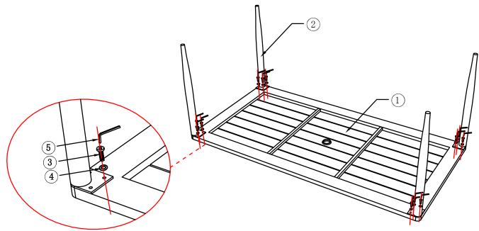
Step 1: Turn the table over and place it on the ground where the exterior finish will not be scratched.
