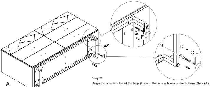
Insert flat washers (D) lock washer (E) and bolt (C) into each hole,
