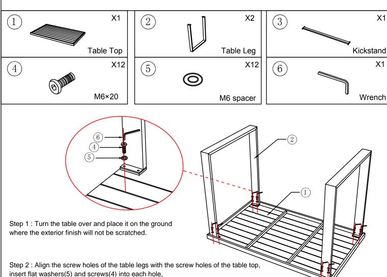
Step 3: Insert the flat washer (5) and screw (4) into each hole, and then install the Kickstand.
